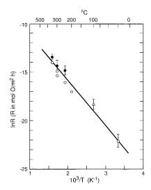
**Fig. 2.** Arrhenius analysis of rate-temperature data for the  $PuO_2 + H_2O$  reaction at 25° to 350°C and 32-mbar  $H_2O$  pressure. Data from MB and PVT measurements are indicated by filled and open circles, respectively. The data point at 100°C (triangle) was determined by using the extent of reaction derived from  $a_o$  of the product and the lattice parameter–composition correlation (Fig. 3). The Arrhenius equation is lnR = -6.441 - (4706/T).
