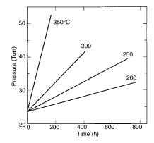
**Fig. 1.** Time dependence of the  $\rm H_2$  pressure during exposure of  $\rm PuO_2$  to  $\rm H_2O$  vapor at experimental temperatures and a constant water pressure of 32 mbar (24 torr).
