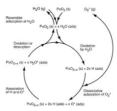
**Fig. 4.** The chemical cycle for  $\rm H_2O$ -catalyzed  $\rm PuO_2 + O_2$  reaction and oxide-catalyzed regeneration of  $\rm H_2O$ .
